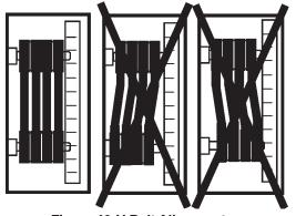
Figure 49. V-Belt Alignment
